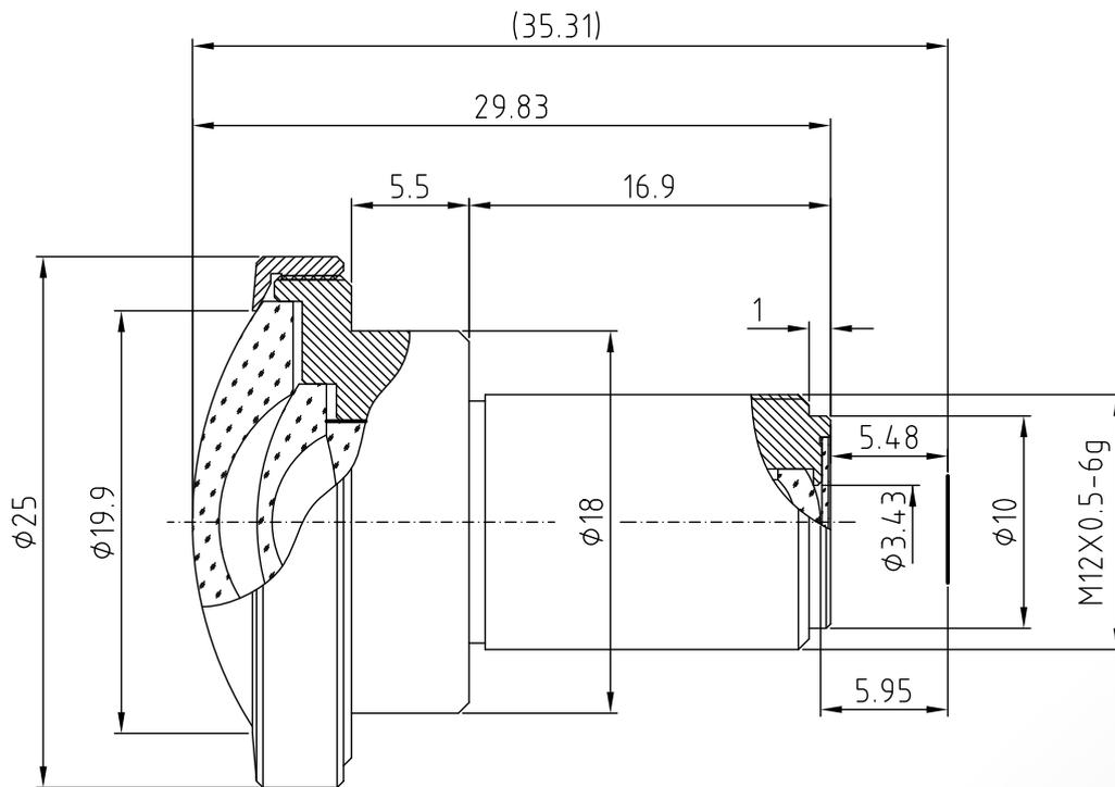
The Fisheye S-Mount lens Lensagon BF5M11920C is suitable for common sensors up to 5 megapixel with an image format of 1/3.2 inch. It is characterized by a particularly high light intensity. Effective Aperture: 19.9mm (Front)
