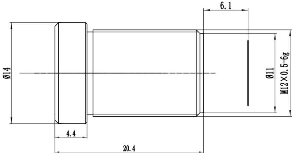
The S-Mount lens Lensagon B5M25024V2 is suitable for common sensors up to 5 megapixel with an image format of 1/2 inch.
