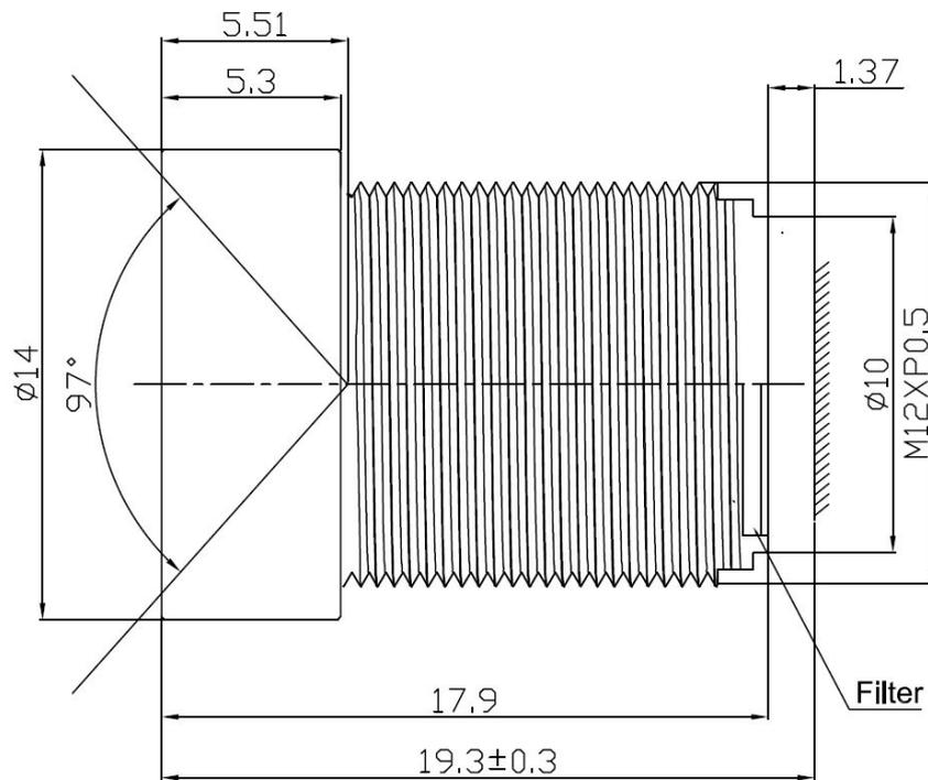
The S-Mount lens Lensagon B3M21835NDC is suitable for common sensors up to 3 megapixel with an image format of 1/4 inch.
