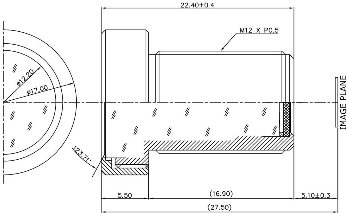
The S-Mount lens Lensagon B2M3814C is suitable for common sensors up to 2 megapixel with an image format of 1/2.5 inch. It is characterized by a particularly high light intensity.
