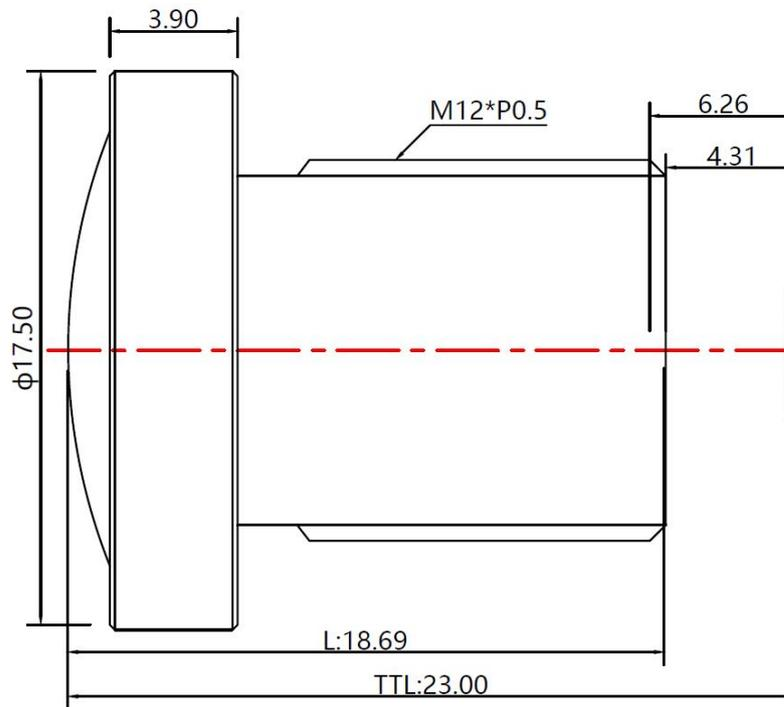
The S-Mount lens Lensagon B14M28620S123 is suitable for current sensors up to 14 megapixel with an image format of 1/2.3 inch.
